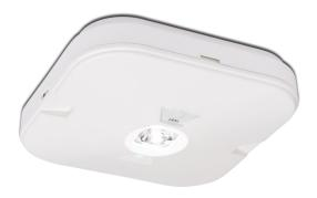
The Luci is a 3 Watt LED surface mounted 3 hour emergency luminaire, with all electronic gear is housed internally within the body. This gives the product a slim minimalist appearance (only 35mm height) without the need to accommodate remote gear.
